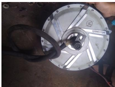
Figure 4. The 3 kW 48 V BLDC motor
