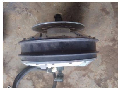
Figure 4. The 3 kW 48 V BLDC motor
